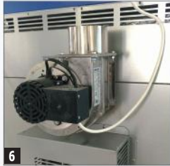
6 Air cooling extractor
