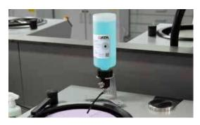
The Qdoser ONE dosing system is an easy-to-use solution for manual or semi-automatic polishing processes. QATM's standard suspension and lubricant bottles can be quickly screwed on the dosing attachment. The dosing volume is closely and continuously controlled with an adjusting screw. The system can be mounted to the polishing heads Qpol GO and ECO. If used with manual grinding/polishing machines, a stand with suction cups can be placed on the machines.
