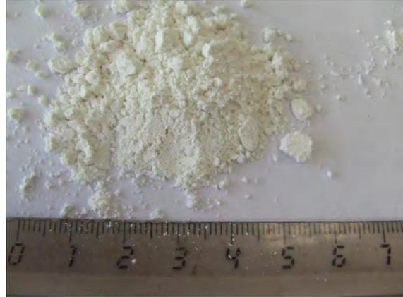
**Fig. 2:** Sample after grinding in the CryoMill
