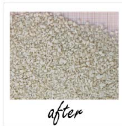
Fig. 3: Degreased human bones before and after grinding in a cutting mill
