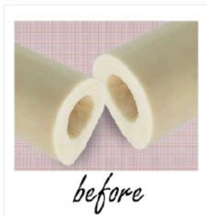
Fig. 3: Degreased human bones before and after grinding in a cutting mill
