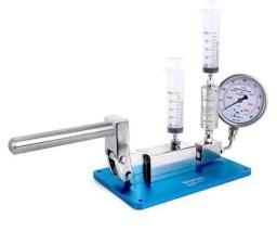
The HandGenizer's mini pump has been designed specifically to provide the preferred pressure to the product stream. When the pump handle is lifted, a small quantity of the sample will be pulled into the mini-pump body. By shifting the pump handle fully down to make a high-pressure profile (maximum 30,000 psi) to the sample stream, this portion of the sample will enter the check valve and the Genizer Y-Type diamond interaction chamber. Finally, it exits the outlet to be collected.
