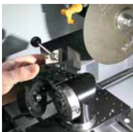
Swivel unit with fast lock vice 50
