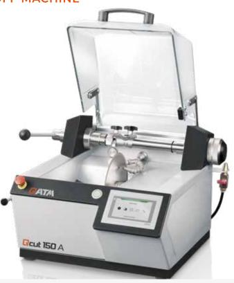
The Qcut 150 A is a compact automatic precision cut-off machine with manual cross feed. With its different operation modes and cooling systems it covers a wide range of applications and materials. The user-friendly system of clamping arm, sample holder and table attachment is designed to change it tool-free. The proven QATM-software on the 4.3" touchscreen contains a consumable and program database which allows also to create individually set user profiles.
