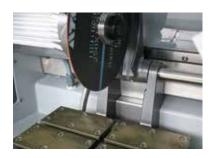
The Qcut 250 M is an especially user-friendly wet abrasive cut-off machine with manual cut-off. Opening the machine folds away the hood to the inside so that the whole cutting chamber is easily accessible. The round window opens a wide field of view during the cutting process.
