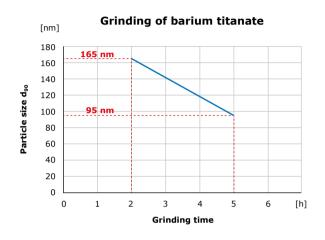
Fig. 2: Result of grinding 110 g barium titanate at 500 min<sup>-1</sup> in the PM 100. After 2 hours of size reduction in 260 ml heptane with 0.5 mm grinding balls, the  $d_{90}$  value of the particle size distribution is 165 nm. By extending the grinding time to 5 h, the  $d_{90}$  value is reduced to 95 nm.
