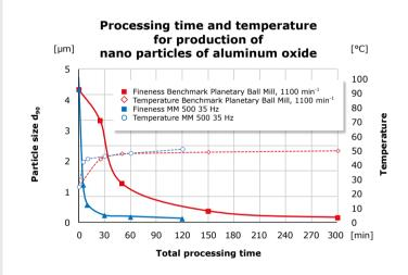
Fig. 2 shows the development of particle fineness and temperature during wet grinding. The MM 500 was operated without cooling breaks, the total process time therefore equals the net grinding time. The MM 500 produced particles of 0.14  $\mu$ m within 2 h net grinding time, whereas 5 h total process time including cooling breaks (1 h net grinding) were required in the Benchmark Planetary Ball Mill to obtain a particle size of 0.18  $\mu$ m.
