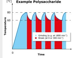
Fig. 4: Grinding of polysaccharide in a defined temperature range between 60 °C and 80 °C. Break times were automatically adjusted by the Emax software.
