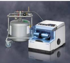
Larger samples of PVC can be pre-cut in a Cutting Mill SM 300 using a 6-disc or a parallel-section rotor and a 6 mm bottom sieve. The granulate resulting from this step can now be pulverized in the CryoMill. Usually, the 50 ml stainless steel grinding jar with one large 25 mm grinding ball, also stainless steel, is suitable to grind about 6 g plastic material. After automatic pre-cooling the sample is pulverized in 9 x 3 min to a final size  $d_{90} = 200 \ \mu m$ .
