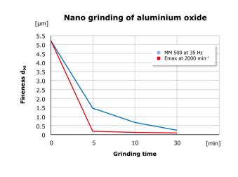
Fig. 3: Nano grinding of aluminum oxide in the Mixer Mill MM 500 and the Emax.
